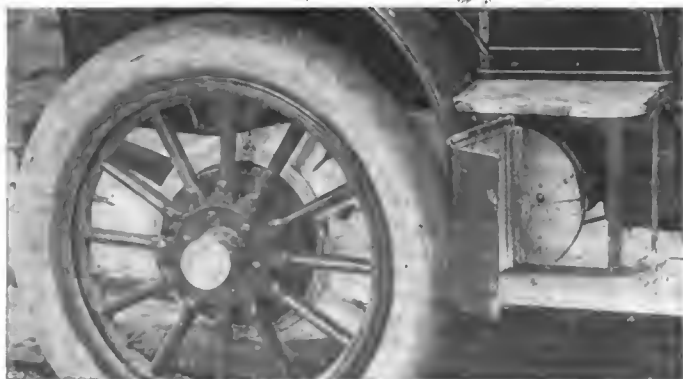
SHOWING THE COMBINED DISTANCE ROD AND CHAIN CASE IN PLACE.
